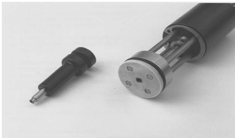
Fig. 3. Close view of the sample cartridges loaded into the vessel's lid.
